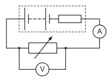
They measure the current and potential difference (p.d.) across the variable resistor for different resistor values.
